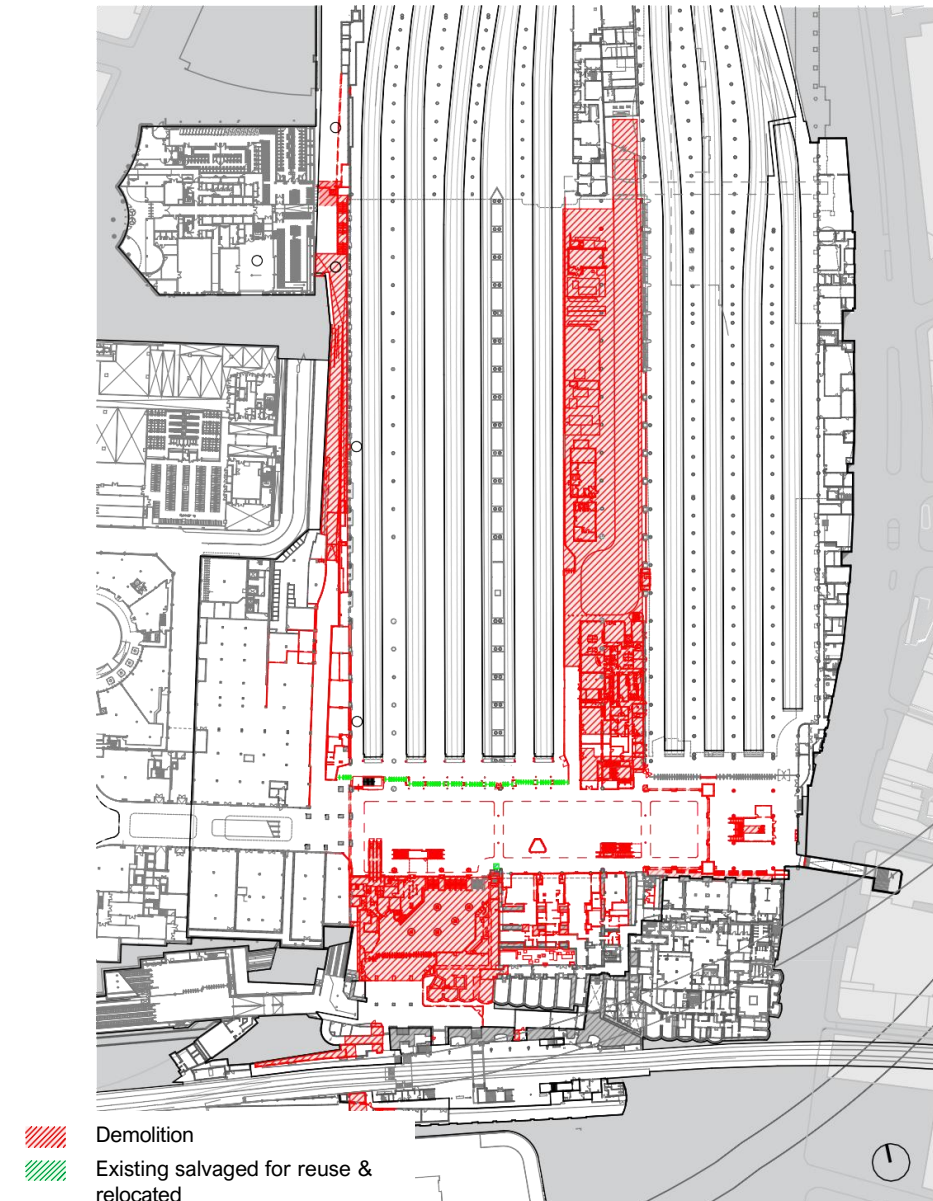
Liverpool Street Station Lower Concourse level plans, existing (left) and demolition (right)
